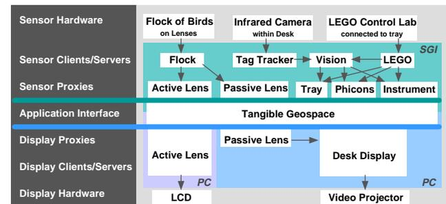
**Figure 10: Tangible Geospace software architecture**
